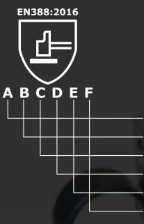
According to this standard, characteristics such as abrasion resistance, cut resistance, tearing strength, puncture resistance and impact protection are tested. In conjunction with the pictogram, four numbers and one or two letters, will be displayed. These signs indicate the performance of the glove.
