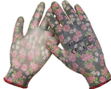
APU512 13 gauge red flower design nylon liner. Knit wrist. White PU coated on palm/finger.
