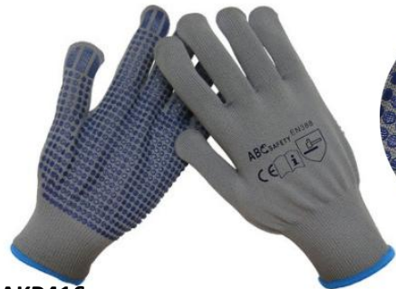
AKP416 13 gauge gray high elastic yarn glove liner, dark blue pvc dots one side, dots diameter 3mm, finger to reinforce the point, gray color rubber band.
