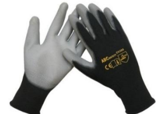
APU117 13 gauge black nylon liner. Knit wrist. Black PU coated on palm/finger.
